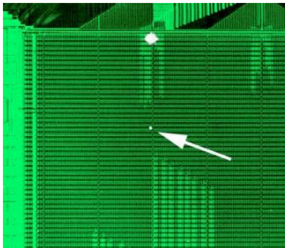
Figure 2 Emission image of the failing cell during program of word line 00 (Bright spot above). The failing cell leaks during program sufficiently to be detected.
