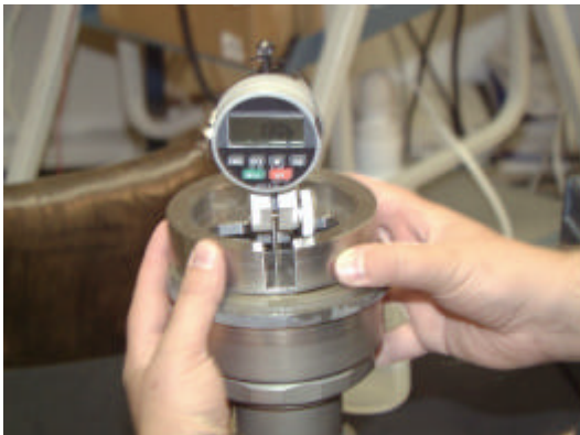
Figure 5. Tilt correction with a micrometer.
