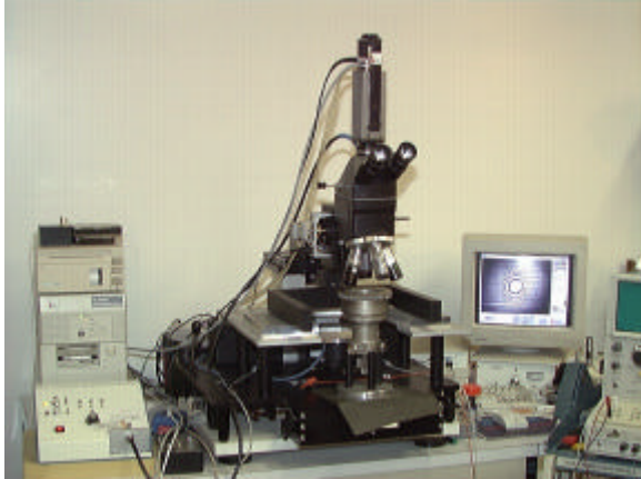
Figure 4. Alpha Innotech Emission microscope setup with the precision polishing jig underneath. A laser illuminator is used to image the sample real time.
