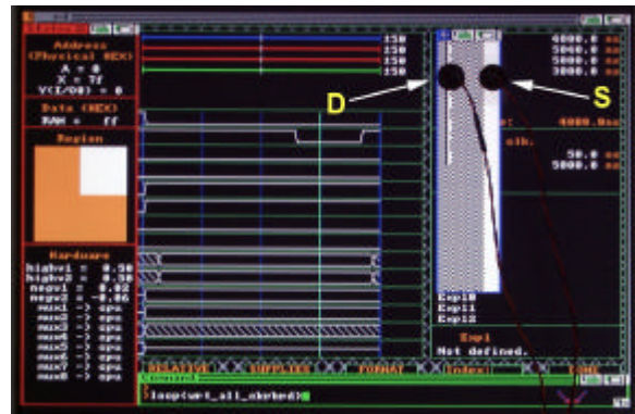
Figure 12. View of the screen on a tester with 2 sensors affixed. The sensor labeled D is the data sensor, which looks for a change in data after sensor S transitions from low to high (strobe).
